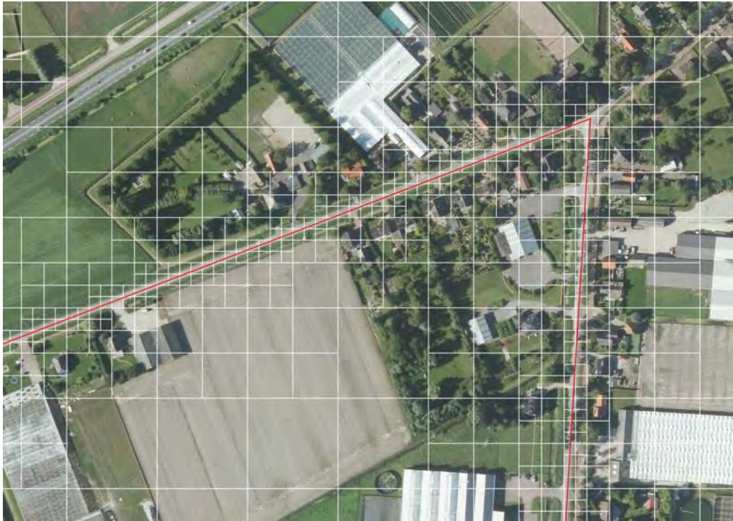
Figure 2: Example of a Quadtree grid (white lines) in combination with obstacles (red line)
