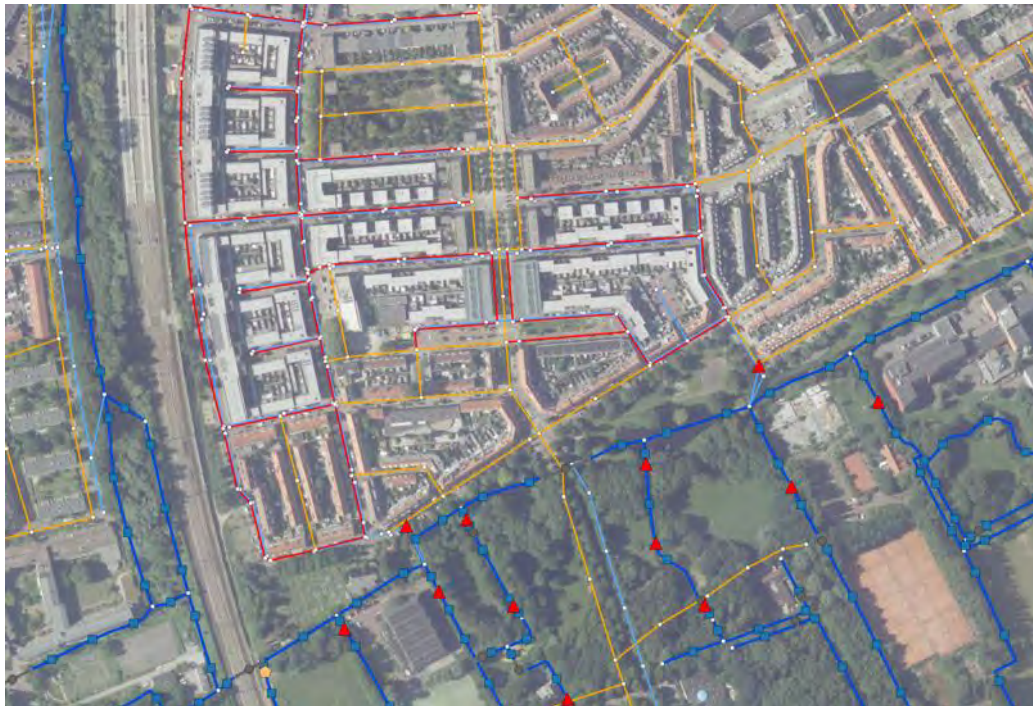
Figure 4: 1D model with surface water (dark blue), mixed (yellow), domestic sewage (red) and rainwater sewage (light blue)
