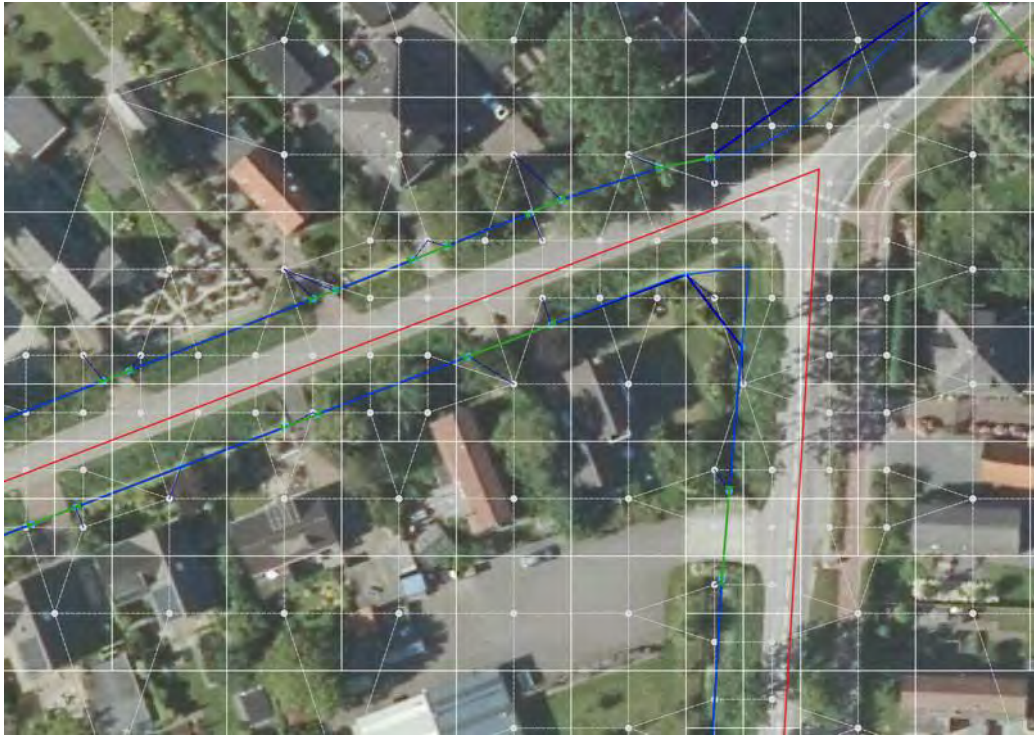
Figure 5: A 2D computing grid (white), coupled via 1D/2D with 1D (open water (blue), combined sewers (green) and dry flow sewage (red))
