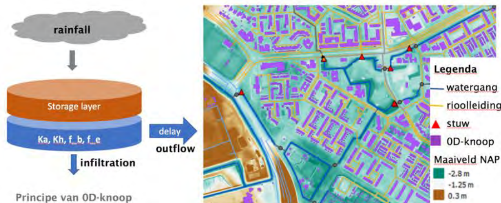
Figure 7: Left, principle of OD node with 6 adjustable parameters per node. Right, detail of a 0D / 1D / 2D model schematic of Rotterdam city
